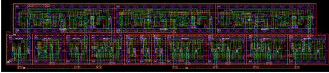
Figure 58: Layout of the digital block from Figure 42. The image shows a  $61\ \mu\text{m}$  by  $12\ \mu\text{m}$  area.
