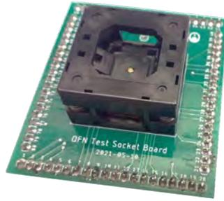
Figure 9: Photograph of the PCB designed to test the second version of the chip.
