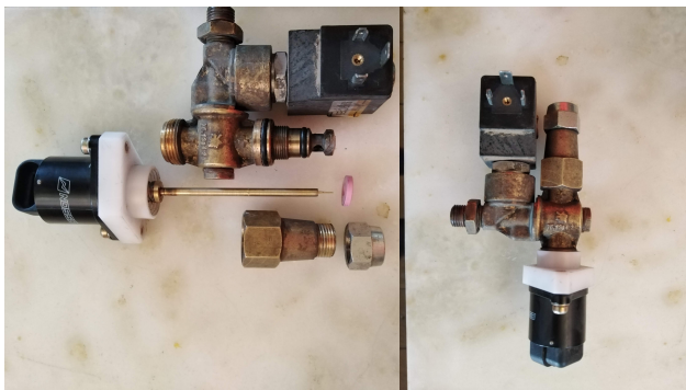
Fig. 6. Implemented nozzle than can vary its flow using a stepper motor. On the left, all the different parts, on the right the ensambled system.
