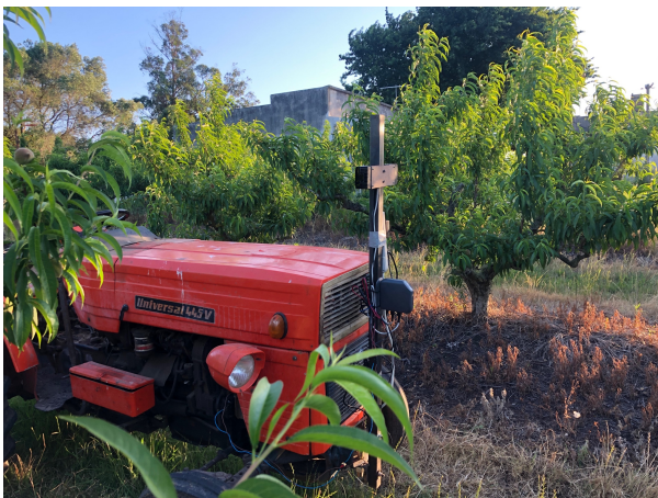
Fig. 3. Sprayer with the LIDARs mounted on the front.
